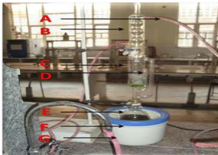
**Figure 3: Soxhlet Apparatus ; A- Water outlet, B- Condenser, C-Thimble, D-Siphon tube, E-Round bottom flask, F-Heating mantle, G- Water inlet.**
